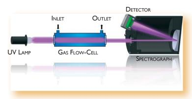
The measuring principle is based on the UV light absorption according to the Beer-Lambert Law:
